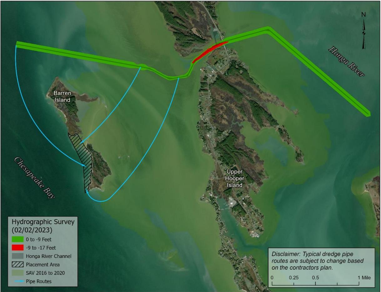
Figure 2 – Hydrographic survey and approximate pipe route options.
